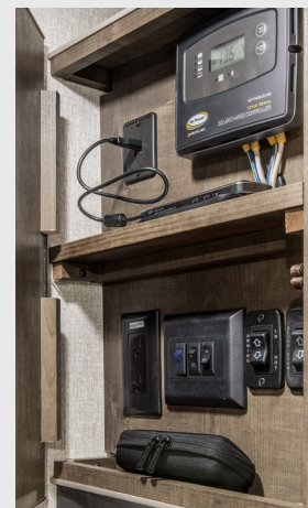
Safe Tek box provides a hidden charging station with USB and 110V outlets. (Sonic & Sonic Lite VBF)
